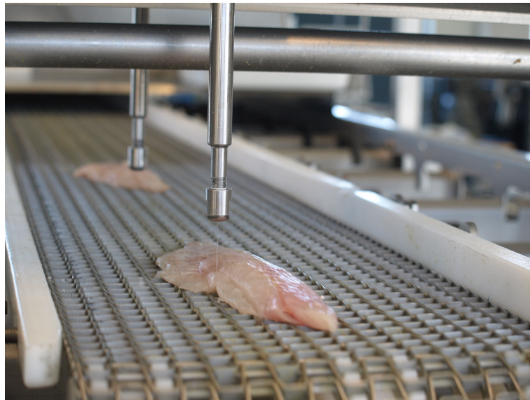
Figure 2.2: [1] The machine that performs the cutting of the fish filets
