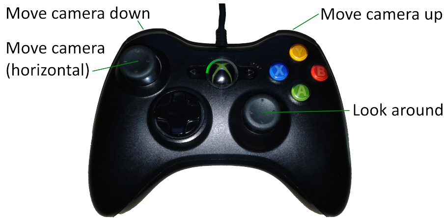
Figure A.1: The controls for the STL viewer and Unprojection viewer.
