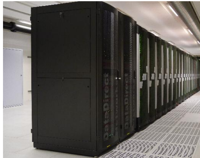
Altix ICE 4800 22464 cores, distributed memory
